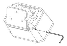
**2. Step:** Fasten the speaker to the wall with 3 screws. Use the correct plugs for the wall.
