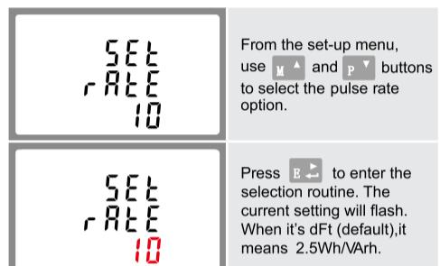
Use **M** and **P** buttons to choose pulse rate, then press **E** to confirm the setting and press **W1** to return to the main set up menu.
