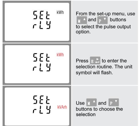
Press **E** to confirm the setting and press **W1** to return to the main set up menu.
