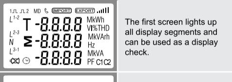
The first screen lights up all display segments and can be used as a display check.
